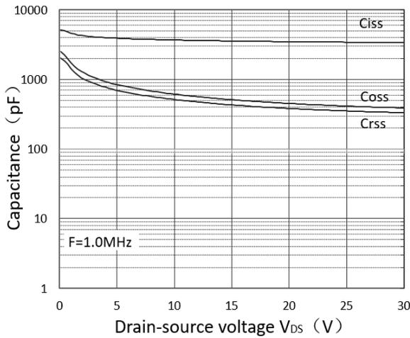
Figure 7. Capacitance Characteristics
