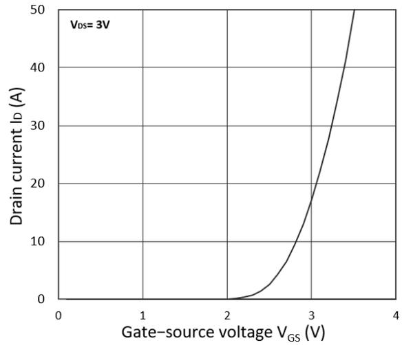
Figure 2. Transfer Characteristics
