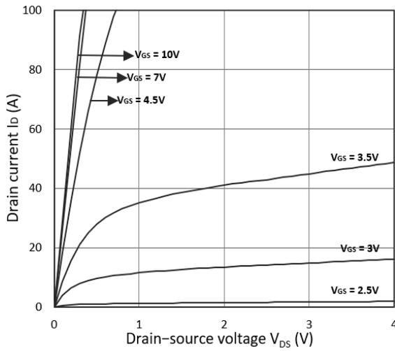
Figure 1. Output Characteristics
